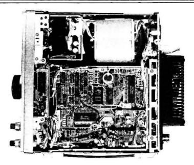
An internal view of the TS-711E which indicates the extent of the circuit integration employed in current transceivers
