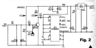
Note: The link should be connected to "a" when using the TTL output and pin 13 grounded using a through-board pin indicated on the p.c.b. layout. For the ECL outputs the link should be connected 'b" and pin 13 left open circuit
