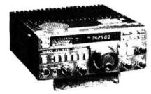
100W multi mode transceiver. Gen. cover. RX, FM & CW narrow, fitted.
