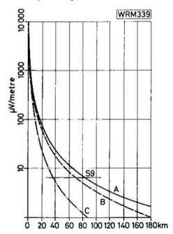
Fig. 8.3: Groundwave field strength at 1-8MHz based on the Sommerfield equation. (A) from a  $\frac{3}{8}$  vertical antenna. (B) from a well elevated horizontal  $\frac{1}{4}$  antenna. (C) from an "L" shaped antenna with most of the horizontal portion at low height. Note: These are for daytime conditions
