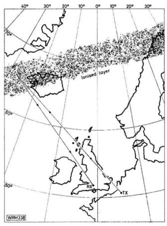
Fig. 8.2: A form of back-scatter allowing communication between two stations a relatively short distance apart but having no direct propagation path to each other. (TX) transmitter (RX) receiver
