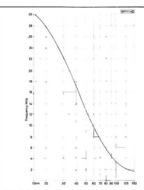
Fig. 8.4: Ground range versus frequency for groundwave propagation. (Daytime conditions 2 to 30MHz)
