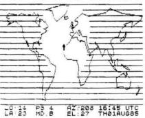
Fig. 2: OSCAR-10 soon after AOS at 1645 August 1 on Mode "B" with satellite just after Perigee, hence small footprint
