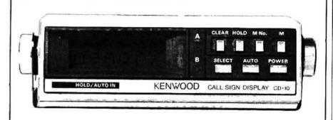
The CD-10 callsign display decodes and displays digital data input as audio. Up to 20 callsigns can be held in its memory or interfaced with your micro for log keeping
